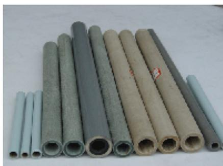
Vulcanized fiber tube is manufactured by winding zinc chloride treated paper on making mandrel to the predetermined wall thickness. Its are then going through puring, drying, rolling, grinding, and sanding processes to get desired inside and outside diameters .It has good physical properties, mechanical properties, dielectric strength, arc resistance, and arc-quenching characteristics.
