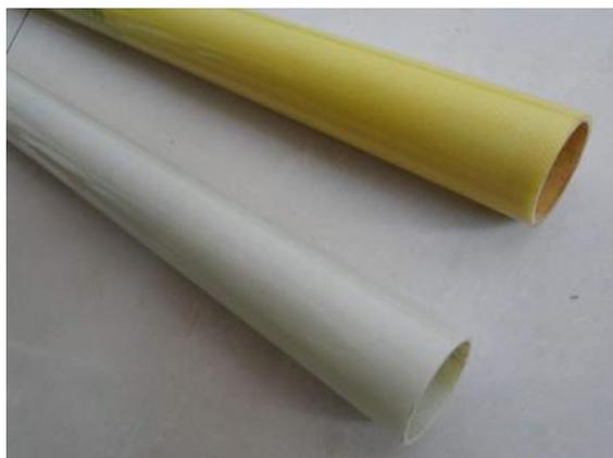
Epoxy fabric tube is formed by high temperature curing of the non-alkali glass fabric impregnated with epoxy resin. With the high mechanical properties, heat resistance and dielectric properties, it is suitable for the electrical equipment as the insulation parts, and may be used in wet conditions and transformer oil..
