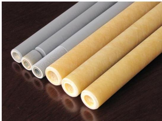
Synthetic liner material fuse tube is new generation of products developed by our company to replace the winding composite tube. Compared with the vulcanized fiber tube fusion tube, there is a qualitative leap in the manufacturing process and product performance. Polymer fusion tube is formed through the curing of a variety of polymer raw materials (partly imported) by a chemical reaction. The hazardous substances such as small molecules
