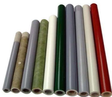
Vulcanized fiber Complex epoxy fiberglass tube from import epoxy resin, fiberglass silk, vulcanized fiber tubes . the fuse tube is fabricated by winding a filament-wound glass-epoxy outer tube over an inner tube of vulcanized fiber that provides the arc-quenching properties.T Fiberglass filaments are wound in two directions across each other and at angle of 50-55 degree to the longitudinal axis of the tube with good tensile and burst strength. Surface: UV resistant insulation Painting.
